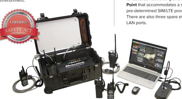
The Compact Go Kit is equipped with a best-in-class portable laptop with speaker/microphone. The kit includes 4 interoperable Radio Gateway ports (radios are not included) and cables, a Video Gateway and an **HDMI** USB converter.
